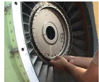
Knowing exactly where to install weights eliminates errors
